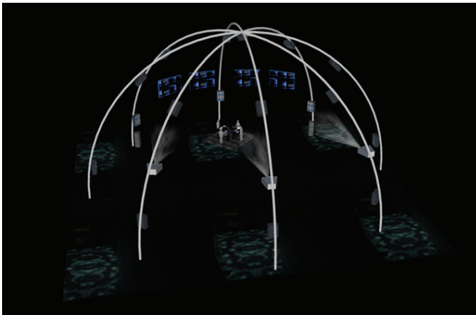
Fig. 2. Dome Multichannel System - 17ch 3D.
